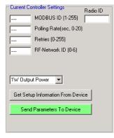
If your system is configured as a Peer to Peer system, the system must consist of one Master and one Slave. The Master controller is responsible for starting the polling sequence.
